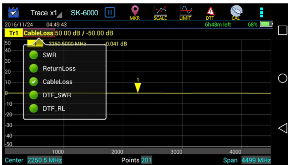
Figure 10 Selecting Cable Loss Measurement
