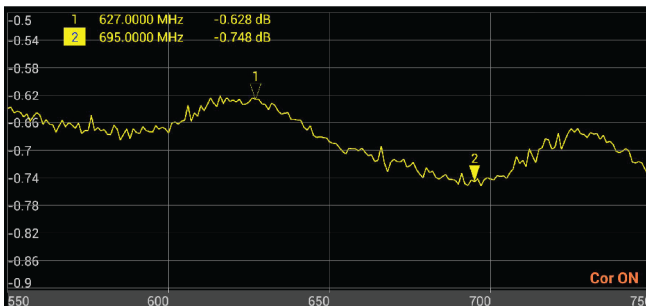
Figure 11 Interpreting Cable Loss Measurement
