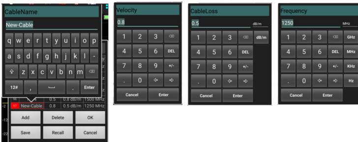
Figure 49 Enter Cable Data
