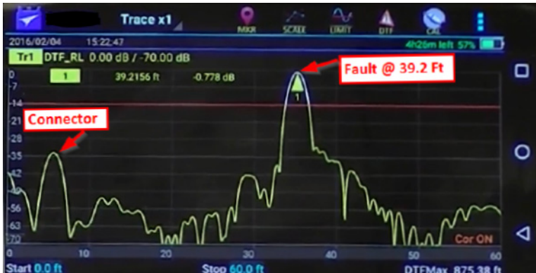
Figure 1 Typical Fault Location Measurement
