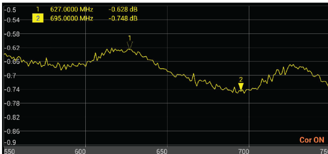
Figure 31 Interpreting Cable Loss Measurement
